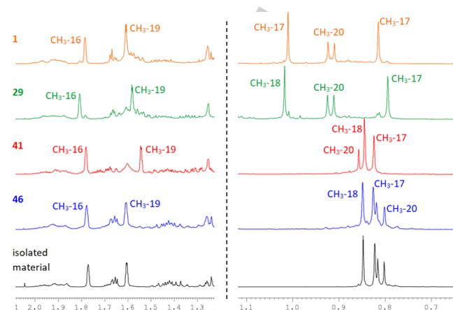
**Figure 3.** Comparison of the <sup>1</sup>H-NMR shifts of the methyl groups of different halioxepine isomers to the one from natural halioxepine.
