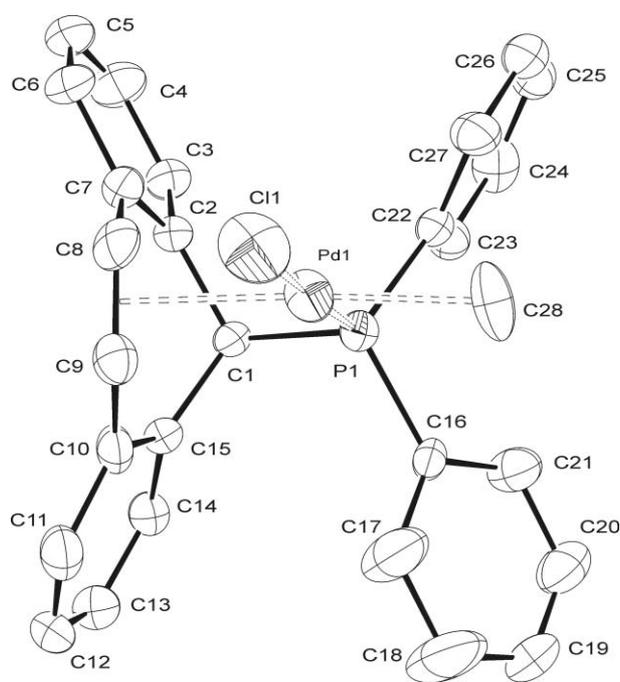
**Fig. 3** ORTEP diagram of **10a**·0.5C<sub>6</sub>H<sub>6</sub> with 30% probability ellipsoids. Hydrogen atoms, the counter-anion and the solvent molecule are omitted for clarity.
