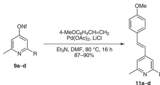
**Scheme 3** Heck–Mizoroki couplings of 4-pyridyl nonaflates **9a–d** leading to (*E*)-4-(4-methoxystyryl)pyridines **11a** ( $R = \text{Me}$ ), **11b** ( $R = \text{Ph}$ ), **11c** ( $R = 2\text{-thienyl}$ ), and **11d** ( $R = 2\text{-furyl}$ )
