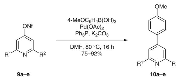
**Scheme 2** Suzuki–Miyaura couplings of 4-pyridyl nonaflates **9a–e** leading to 4-(4-methoxyphenyl)pyridines **10a** ( $R^1 = \text{Me}$ ,  $R^2 = \text{Me}$ ), **10b** ( $R^1 = \text{Me}$ ,  $R^2 = \text{Ph}$ ), **10c** ( $R^1 = \text{Me}$ ,  $R^2 = 2\text{-thienyl}$ ), **10d** ( $R^1 = \text{Me}$ ,  $R^2 = 2\text{-furyl}$ ), and **10e** ( $R^1 = \text{Ph}$ ,  $R^2 = \text{Ph}$ )
