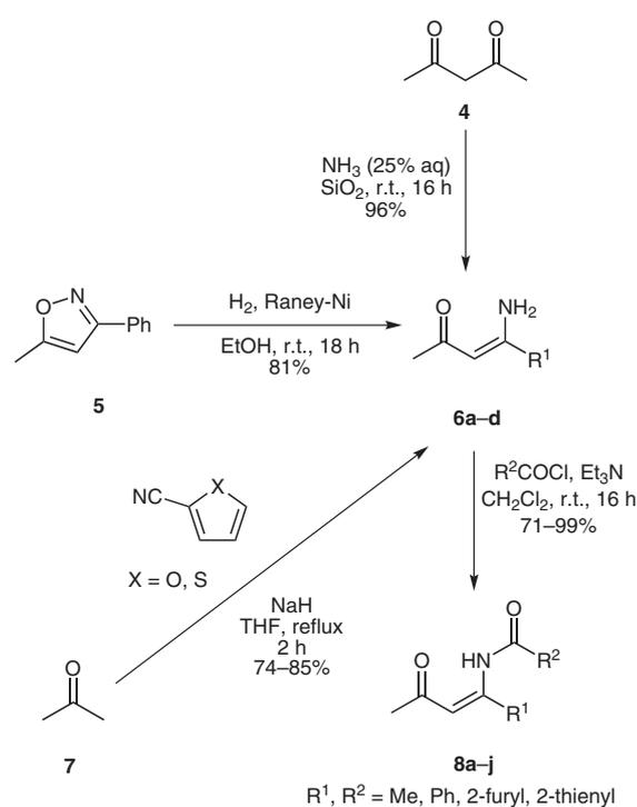
**Scheme 1** Preparation of  $\beta$ -ketoenamides **6a** ( $R^1 = \text{Me}$ ), **6b** ( $R^1 = \text{Ph}$ ), **6c** ( $R^1 = 2\text{-thienyl}$ ), and **6d** ( $R^1 = 2\text{-furyl}$ ) and  $\beta$ -ketoenamides **8a–j** (for substituents  $R^1$  and  $R^2$  of compounds **8**, see Table 1)
