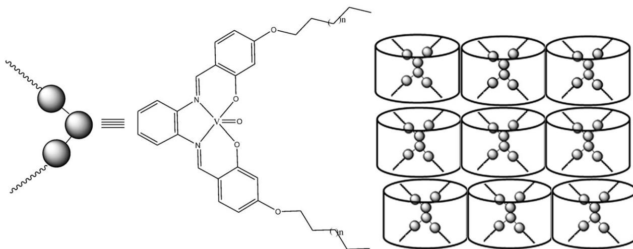
Fig. 5. Antiparallel arrangement of molecules in the lamellar columnar mesophase.
