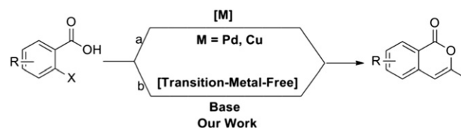
Scheme 1. Transition-metal catalyzed or base-promoted cyclization reaction of corresponding 2-iodobenzoic acid.
