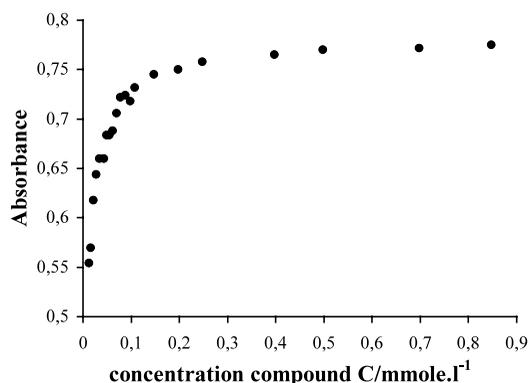
Fig. 7. CMC determination of compound C by Menger and Portnoy method, absorbance measurement at 610 nm and 25 °C of an  $1.10^{-6}$  M aqueous pinacyanol chloride solution with variable surfactant concentrations.
