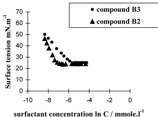
Fig. 6. Plots of surface tension at 25 °C in water vs. ln concentration of cosurfactants **B2** and **B3**.
