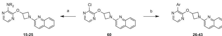
**Scheme 2.** Reagents and conditions: (a) secondary amine, K<sub>2</sub>CO<sub>3</sub>, *i*PrOH/water, μW, 160 °C, 5 h; (b) ArB(OH)<sub>2</sub>, Pd(PPh<sub>3</sub>)<sub>4</sub>, Na<sub>2</sub>CO<sub>3</sub>, dioxane/water, 110 °C or, for example **33**, Pd(PPh<sub>3</sub>)<sub>4</sub>, 2-tributylstannyl-pyridine, toluene, 110 °C.
