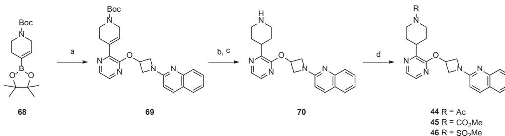
**Scheme 4.** Reagents and conditions: (a) intermediate **60**, Pd(dppf)Cl<sub>2</sub>, K<sub>3</sub>PO<sub>4</sub>, dioxane/H<sub>2</sub>O (b) Pd/carbon, H<sub>2</sub>, MeOH, rt; (c) HCl, MeOH, rt; (d) RCl, Et<sub>3</sub>N, DCM, 0 °C.
