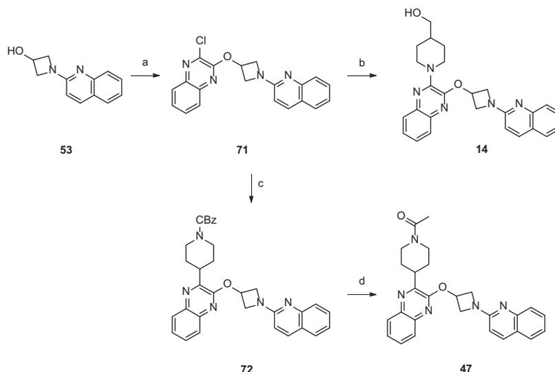
**Scheme 5.** Reagents and conditions: (a) 2,3-dichloroquinoxaline, NaH, DMF, 90 °C; (b) 4-piperidinemethanol, K<sub>2</sub>CO<sub>3</sub>, iPrOH/H<sub>2</sub>O,  $\mu$ W, 160 °C, 5 h; (c) benzyl 4-iodopiperidine carboxylate, zinc, TMSCl, 1,2-dibromoethane, PdCl<sub>2</sub>dppf, CH<sub>2</sub>Cl<sub>2</sub>, CuI, DMA, 80 °C; (d) H<sub>2</sub>, Pd(OH)<sub>2</sub>, Ac<sub>2</sub>O, toluene, rt.
