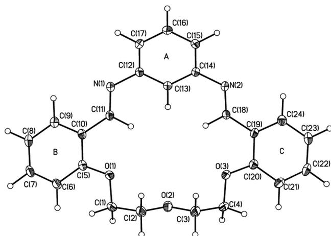
**Figure 1.** Molecular structure of compound **2b** with atoms represented as thermal vibration ellipsoids of 50% probability.
