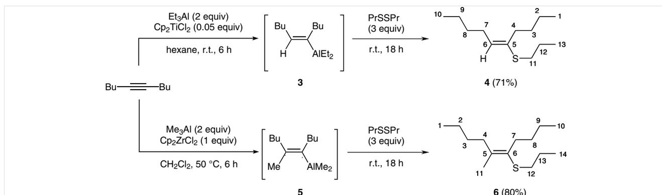
**Scheme 1** Preparation of alkenyl sulfides **4** and **6** from dec-4-yne
