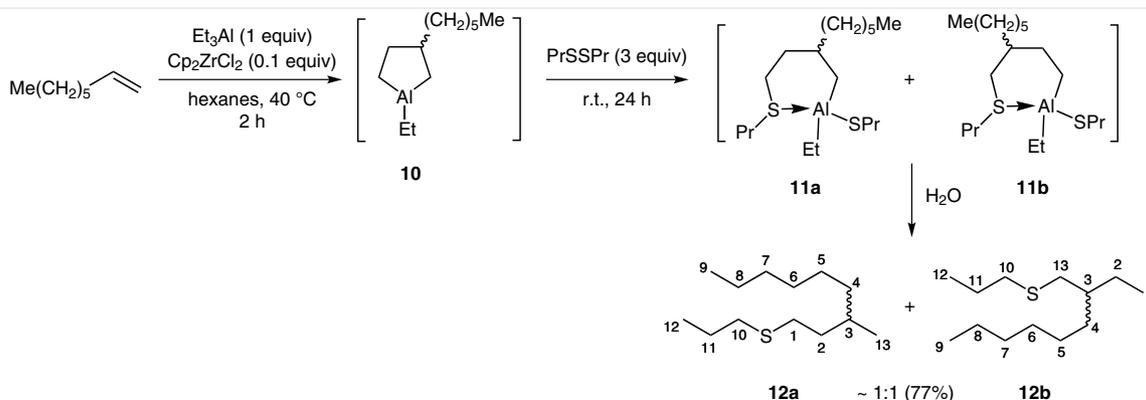
**Scheme 3** Preparation of dialkyl sulfides **12** from oct-1-ene
