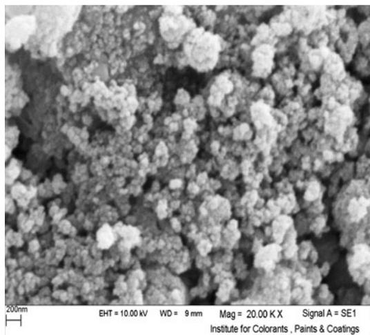
**Fig. 2** SEM image of the FeCl<sub>3</sub>/SiO<sub>2</sub> NPs
