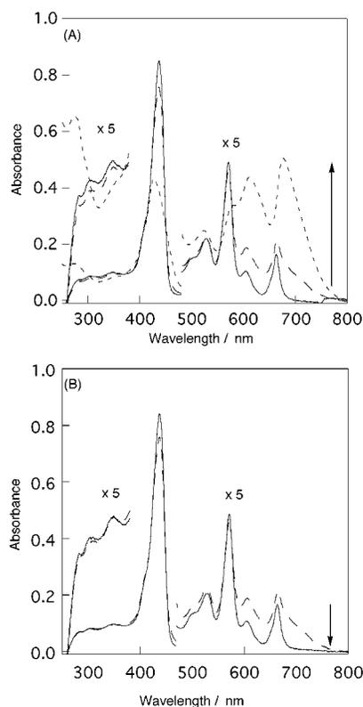
**Figure 8.** Photoisomerization of **6** in THF. A, top, open-to-closed starting from pure open form (—); photostationary state for excitation at 330 nm (---) and pure closed form (· · ·). B, bottom, closed-to-open starting from the photostationary state (—); photostationary state for excitation at >550 nm (---).
