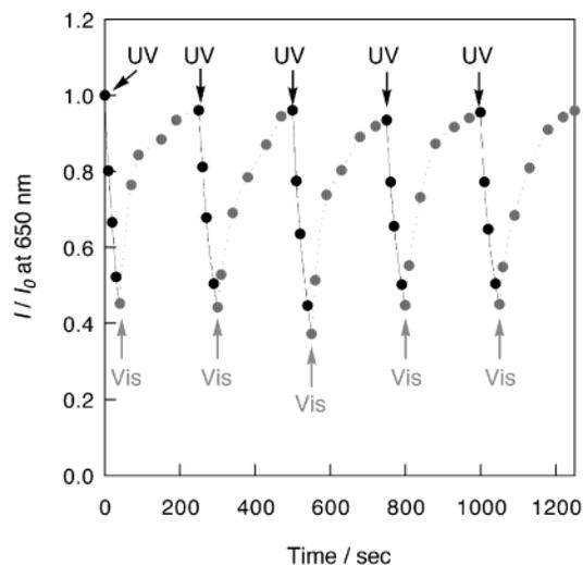
**Figure 7.** Fluorescence intensity changes of **4** at 650 nm upon photoirradiation at 330 nm (UV) and  $>550$  nm (vis) taken for excitation at 430 nm.
