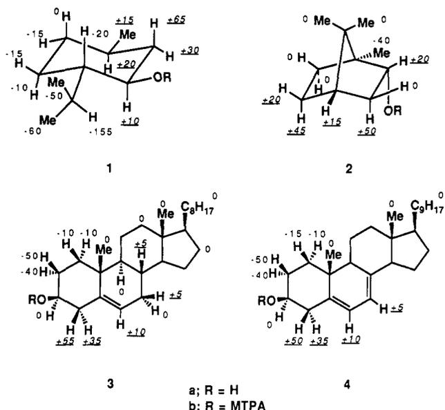
**Figure 2.**  $\Delta\delta$  values obtained for the MTPA esters of (-)-menthol (**1a**), (-)-borneol (**2a**), cholesterol (**3a**), and ergosterol (**4a**).  $\Delta\delta$  values are expressed in hertz (500 MHz).
