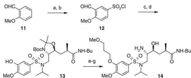
**Scheme 2.** Reagents and conditions: (a) HC(OEt)<sub>3</sub>, NH<sub>4</sub>Cl, EtOH, reflux, 90%. (b) ClSO<sub>3</sub>H, 3 h at -5 °C, then 2 h at rt, 80%; (c) **8**, DIEA, CH<sub>2</sub>Cl<sub>2</sub>, 0 °C, 16 h, 72%; (d) MCPBA, CHCl<sub>3</sub>, 48 h, rt; then Et<sub>3</sub>N, MeOH, rt, 2 d, 55%. (e) MeO(CH<sub>2</sub>)<sub>3</sub>I, K<sub>2</sub>CO<sub>3</sub>, MeCN, reflux, 18 h, 82%. (f) CSA, MeOH, rt, 89%; (g) 4 N HCl-dioxane, 0 °C, 2 h, 82%.
