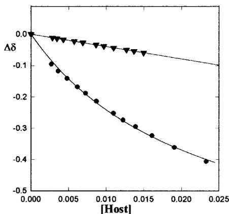
**Figure 3.** Titration of ACh iodide with host **1** (▼) and host **2a** (●)  $NCH_3$  protons. Points are experimental and curves are calculated
