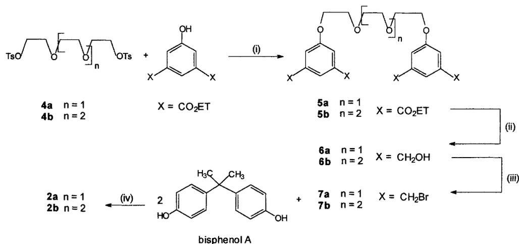
**Scheme 1.** Synthesis of cyclophanes **2a** and **2b**. (i)  $\text{K}_2\text{CO}_3$ ,  $\text{CH}_3\text{CN}$ ; (ii)  $\text{LiAlH}_4$ , THF; (iii)  $\text{PBr}_3$ , dioxane; (iv)  $\text{KOH}$ , DMSO, high dilution
