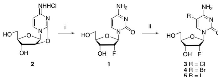
**Scheme 1.** Reagents and conditions: (i) KF, dibenzo[18]crown-6, DMF, 120 °C, 4 h; (ii) BzCl, *m*-CPBA, DMF, rt, 30 min; or pyridine, Br<sub>2</sub>, CCl<sub>4</sub>, rt, 25 min; or MeOH, ICl, 50 °C, 4 h.
