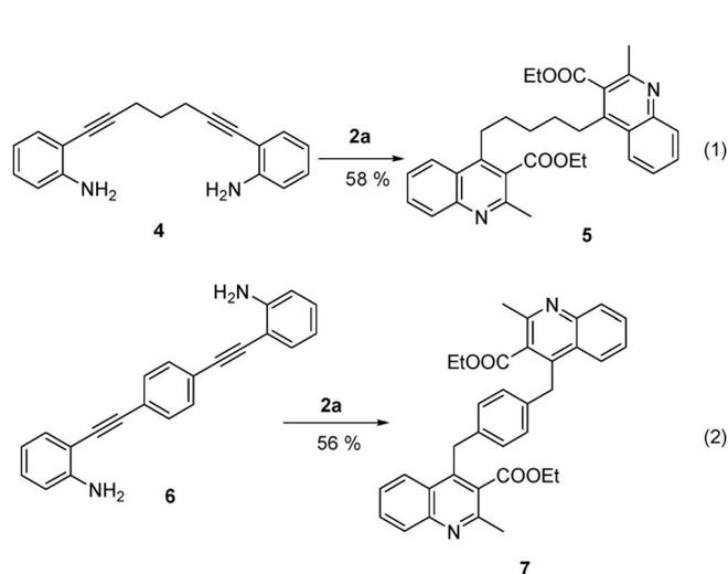
Scheme 2. Synthesis of dimeric quinolines with alkyl or aryl linkages at C-4.
