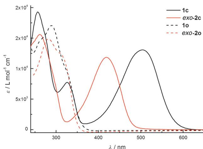
**Figure 2.** Comparison of the absorption spectra of **1o**, **1c**, *exo-2o*, and *exo-2c* in acetonitrile at 25 °C. The residual absorbance of *exo-2c* above 500 nm is attributed to a minor retro DA reaction taking place during the irradiation process.
