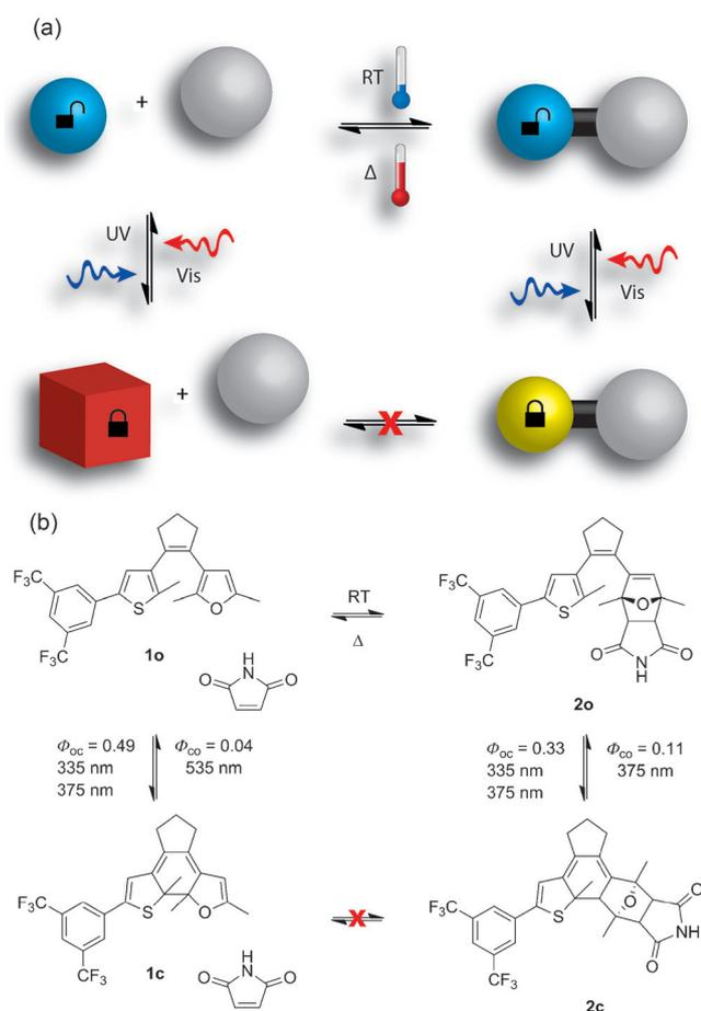
**Scheme 1.** Photocontrol over the formation and scission of a dynamic bond using photoswitches as locks. a) Concept. b) The different components **1o**, **1c**, **2o**, **2c**, and maleimide in the course of a photocontrolled Diels–Alder reaction, with the respective photocyclization and ring-opening quantum yields measured in toluene as well as the irradiation wavelengths employed for the in situ reaction.
