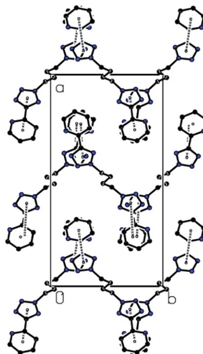
**Figure 3.** Crystal packing of **3m**, viewed along the  $c$  axis. The methyl groups and hydrogen atoms are omitted for clarity. Dashed lines show  $\pi$ - $\pi$  stacking interactions.
