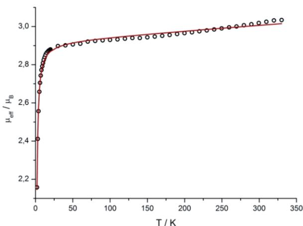
**Figure 7.** Temperature dependence of  $\mu_{\text{eff}}$  for  $[Cu_2(bpt)Cl_4]$  (o) per dinuclear unit. The solid red line represents the best theoretical fit [Equation (1)].
