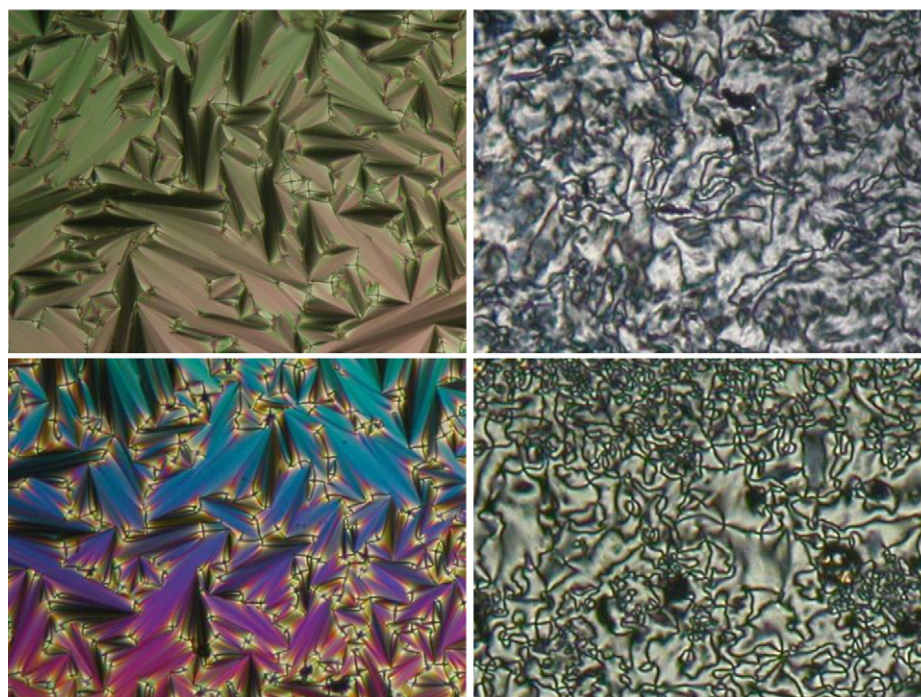
Fig. 1. Optical textures observed. Top left and right plates: SmA phase at 360.0 °C and SmC phase at 340.0 °C by 1a ( n=8 ). Bottom left and right plates: SmA phase at 320 °C and SmC phase at 312.0 °C by 1a ( n=14 ).
