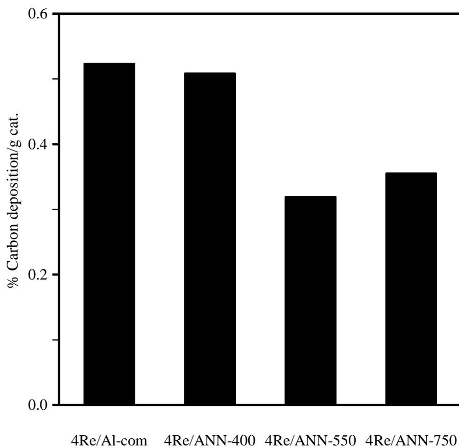
**Figure 9** The amount of coke deposit on the spent catalysts
