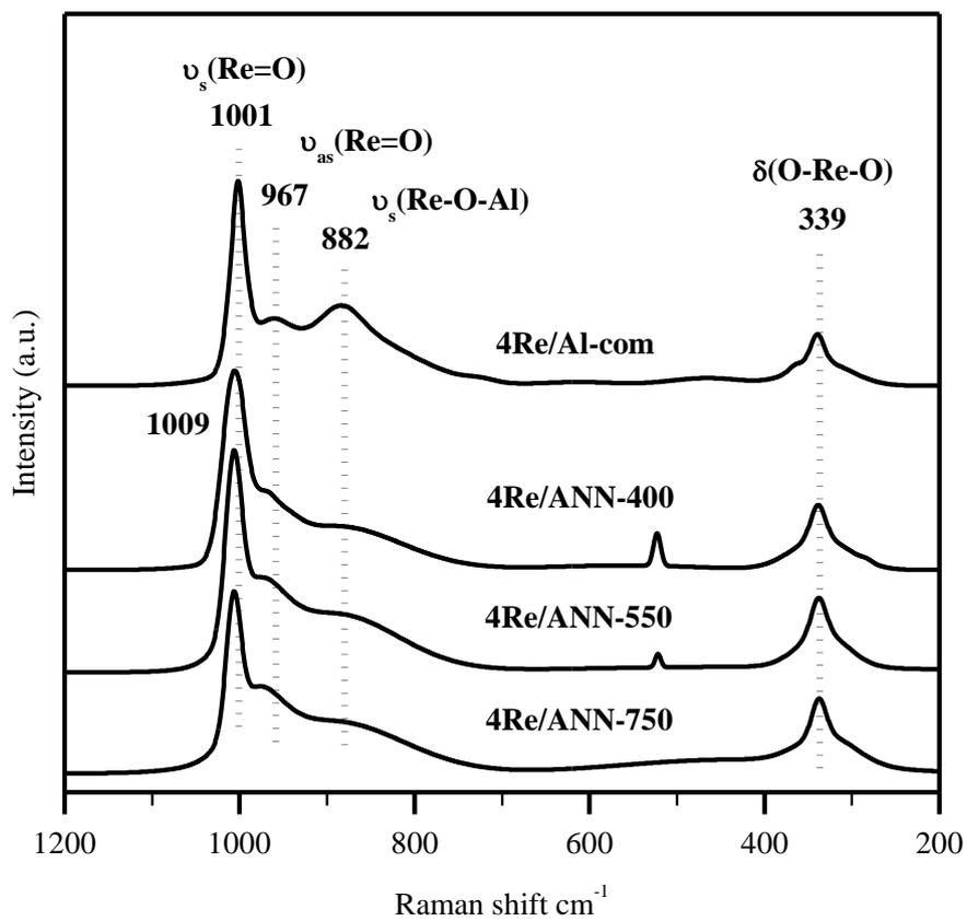
**Figure 3** In situ Raman spectra of catalysts under dehydrated condition at 60 °C
