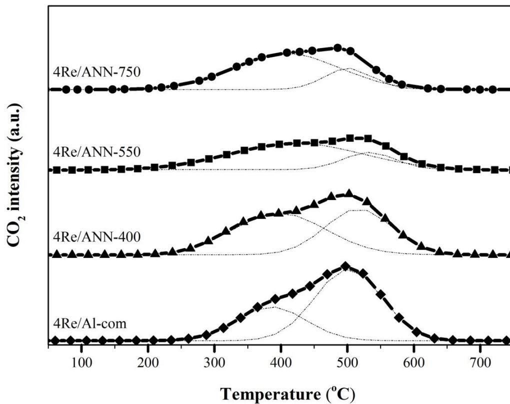
**Figure 10** Temperature programmed oxidation (TPO) patterns of the spent catalysts
