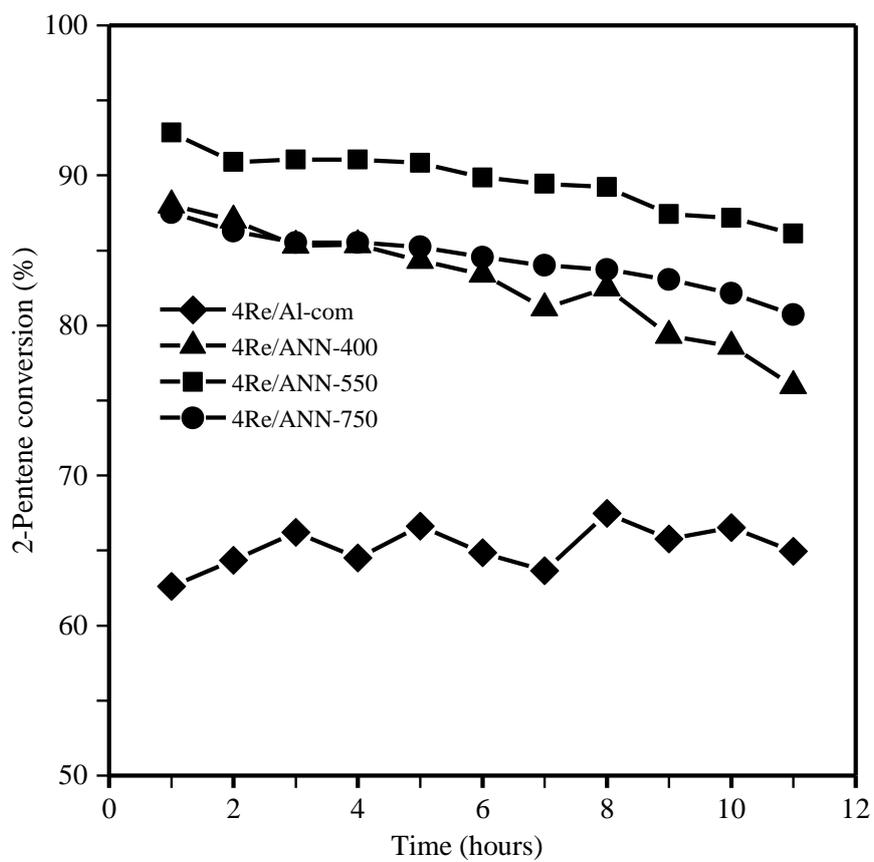
**Figure 6** The 2-pentene conversion of the prepared catalysts over the metathesis reaction as a function of reaction time
