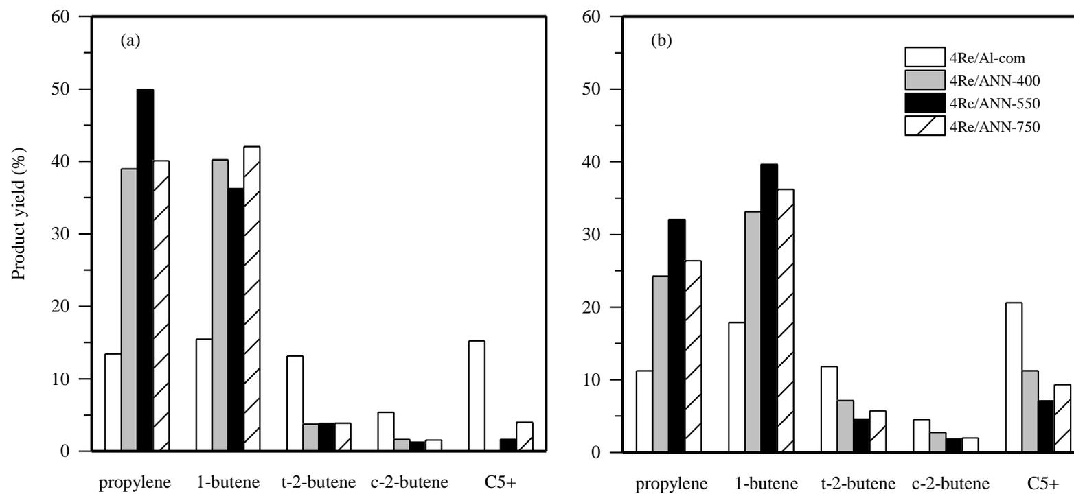
**Figure 7** Product distributions of different catalysts at (a) 1 h and (b) 11 h reaction time
