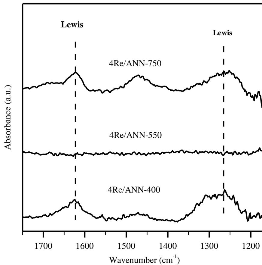
**Figure 5** In situ IR subtracted spectra of chemisorbed ammonia over the catalysts at 250 °C
