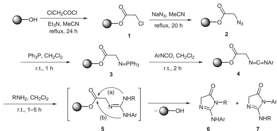
**Scheme 1** Synthesis of imidazolin-4-ones **6** or **7** using poly(ethylene glycol) as soluble support
