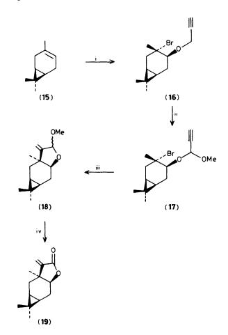
Scheme 3. Reagents and conditions: i,  $HC\equiv CCH_2OH$ , NBS; ii,  $Bu^tOK$  (cat. amount), pentane, room temp.; iii,  $Bu_3SnH$ , AIBN,  $C_6H_6$ ; iv,  $m\text{-}ClC_6H_4CO_3H$ ,  $BF_3\text{-}Et_2O$ .
