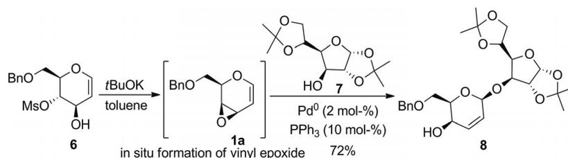
Scheme 2. Glycosylation of vinyl oxirane **1a** with diacetone-*D*-glucose by using  $Pd^0$  catalyst.
