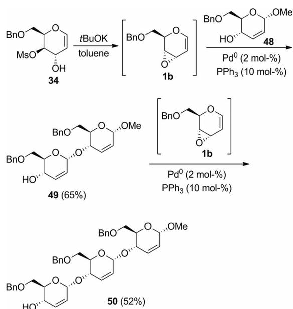
Scheme 7. Stereoselective synthesis of trisaccharide **50** by using a  $\text{Pd}^0$  catalyst.
