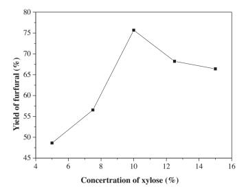
**Figure 3.** Effect of changing initial concentration of xylose on furfural yield under the following conditions: 150 mL of toluene, 10 mL of an aqueous solution of 10%  $H_2SO_4$  (w/w), 1.2 g NaCl, heating for 5 h.
