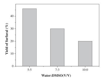
**Figure 5.** Effect of DMSO content in water/DMSO (V/V) mixture on yield of furfural under the following conditions: 150 mL of toluene, 10 mL of an aqueous solution of 10% xylose (w/w), 10%  $H_2SO_4$  (w/w), 1.2 g NaCl, heating for 2 h.
