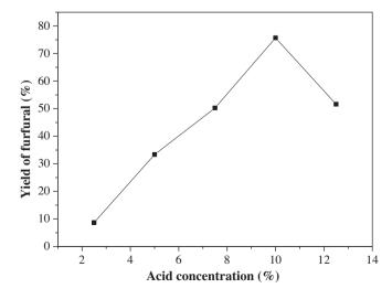
**Figure 2.** Yield of furfural at different sulfuric acid concentrations under the following conditions: 150 mL of toluene, 10 mL of an aqueous solution of 10% xylose (w/w), 1.2 g NaCl, heating for 5 h.
