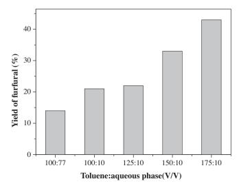
**Figure 1.** Effect of the toluene-to-aqueous phase ratio (V/V) on the furfural yield under the following conditions: 10% xylose (w/w), 5% H<sub>2</sub>SO<sub>4</sub> (w/w), 1.2 g NaCl, heating for 5 h.
