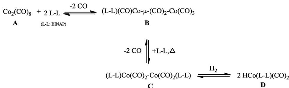
**Scheme 1.** Equilibria found with the system  $\text{Co}_2(\text{CO})_8/\text{L-L}/\text{H}_2/\text{CO}$ .
