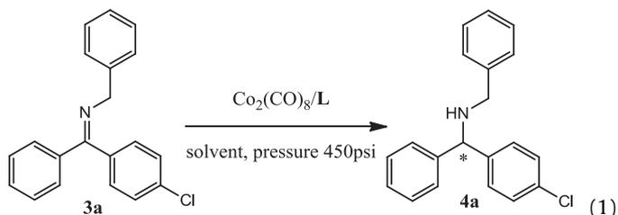
At room temperature, the hydrogenation product was not observed (entry 5) but, a temperature increase (120 °C) favored conversion and reaction yields (entries 4 and 6). The use of a coordinating solvent (THF) led to the best enantiomeric excess (95%ee) (entry 11), that contrasts with lower values obtained when carrying out the reaction in other solvents such as: toluene (67%ee), benzene (75%ee) and methylene chloride (52%ee) (entries 8–10).
