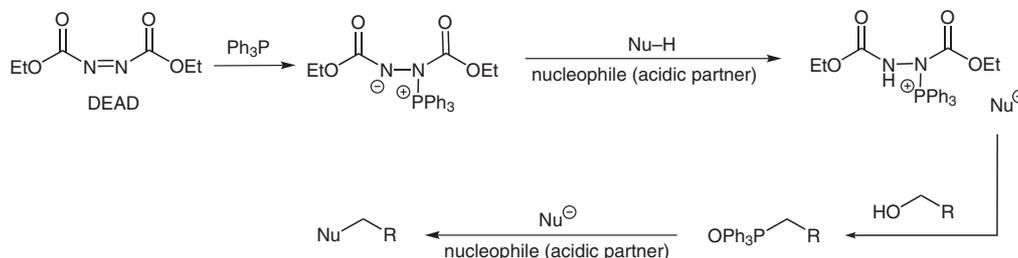
Scheme 1 Mitsunobu reaction pathway<sup>9</sup> under standard conditions.  $pK_a$  of nucleophile must be less than 11 to allow deprotonation step to occur
