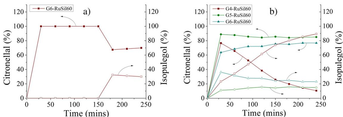
**Fig. 2.** Selectivity observed for the citral hydrogenation reaction using the RuSil60 catalysts at a) 110 °C while evaluating G6-RuSil60 and b) 130 °C when evaluating G4-RuSil60, G5-RuSil60 and G6-RuSil60.
