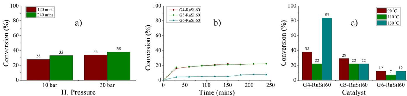
**Fig. 1.** Conversion of citral illustrated for a) pressure dependant conversion of citral at 120 min and 240 min for a H<sub>2</sub> pressure of 10 bar and 30 bar using the G4-RuSil60 catalyst, and conversion of citral using the various RuSil60 catalysts and at various temperatures illustrated by the b) time-resolved conversion of citral at 110 °C and c) end of run conversion of citral at 90 °C, 110 °C and 130 °C.
