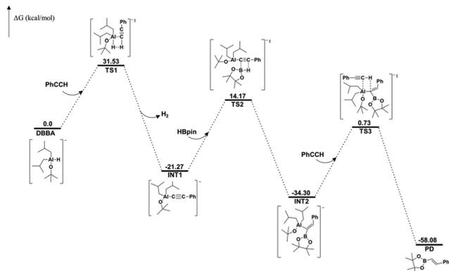
**Scheme 5** Free energy profile (in kcal mol<sup>-1</sup>) for LDBBA catalyzed hydroboration of phenylacetylene. (Note: To avoid complications in the calculations, the effect of the Li atom on the energy profile was not taken into account, LDBBA is mentioned as DBBA).
