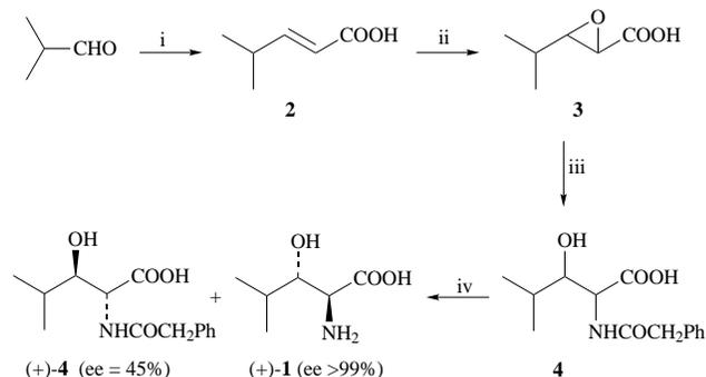
**Scheme 1** Reagents and conditions: i, CH<sub>2</sub>(COOH)<sub>2</sub>, pyridine, 0 °C, 2 h, 80 °C, 8 h, 80%; ii, Oxone, acetone, NaHCO<sub>3</sub>, 24 °C, 2 h, 98%; iii, aq. NH<sub>3</sub>, reflux, 6 h, PhCH<sub>2</sub>COCl, OH<sup>-</sup>, 0 °C, 2 h, 95%; iv, immobilized penicillin G acylase, pH 7.8–8.0, 1 h, 40% conversion, 71% of theoretical yield
