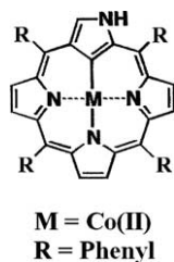
Scheme 1. Schematic structure of Co(II)NCTPP.
