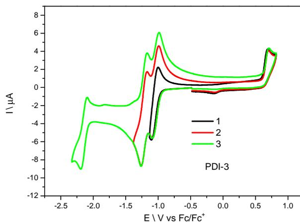
**Fig. 4.** Cyclic voltammograms for **PDI3**. CV sweep rate  $v = 100$  mV/s, 0.1 M  $Bu_4NPF_6$  in  $CH_2Cl_2$  with different lower vertex potential.
