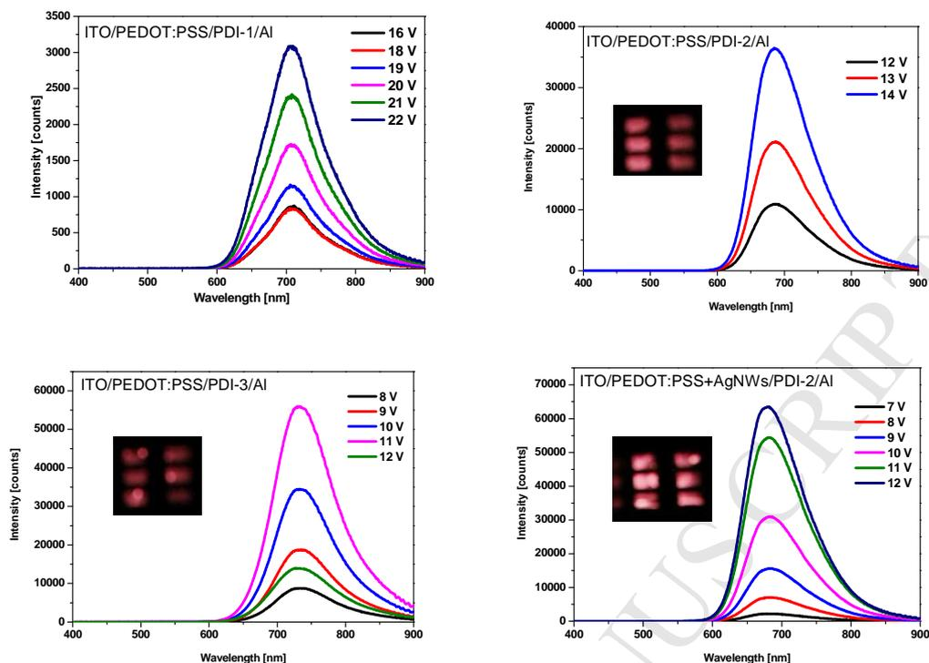
**Fig. 2.** Electroluminescence spectra of fabricated diodes as a function of the applied voltage.
