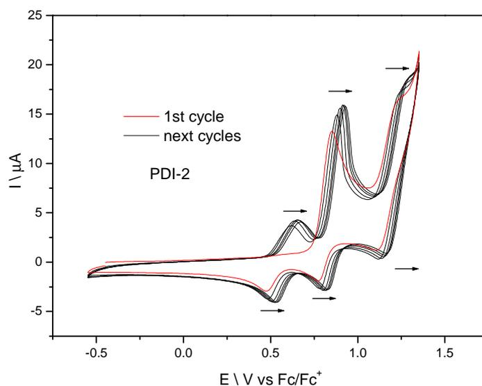
**Fig. 5.** Cyclic voltammograms for **PDI2**. CV sweep rate  $v = 100$  mV/s, 0.1 M  $Bu_4NPF_6$  in  $CH_2Cl_2$ . Arrows indicate shifts in peak maxima.
