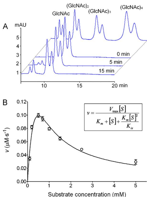
**Fig. 1.** Substrate inhibition of OfHex1. (A) HPLC analysis of hydrolysis products using (GlcNAc)<sub>2</sub> as substrate in the presence of OfHex1. (B) Nonlinear fitting of the substrate pNP-β-GlcNAc concentration vs. velocity plot to the equation of 'second substrate binding'. The experimental data were indicated by open circles and the fitted curve was indicated by lines.
