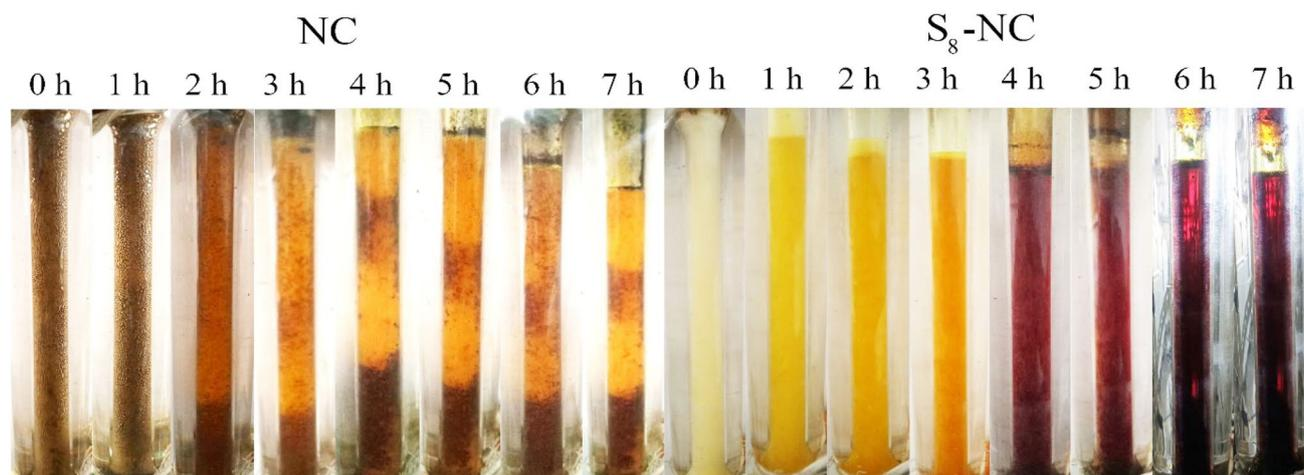
**Fig. 3** Pictures of the bubble column reactor at different times during the reaction
