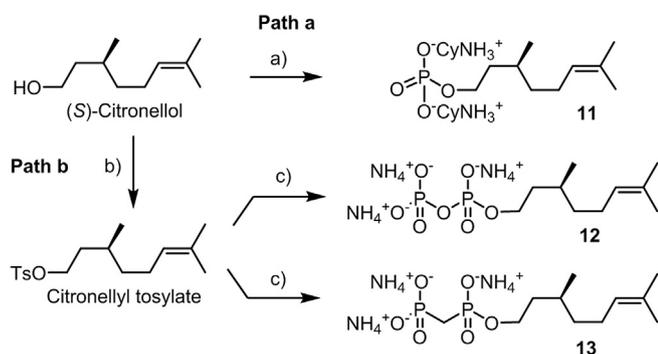
**Scheme 2.** a)  $\text{POCl}_3$ ,  $\text{Et}_3\text{N}$ ,  $\text{CH}_2\text{Cl}_2$ , RT, 1 h, then acetone/ $\text{Et}_3\text{N}$ /water, RT, 14 h, recrystallization with cyclohexylamine, 33%. b)  $\text{TsCl}$ ,  $\text{DMAP}$ ,  $\text{CH}_2\text{Cl}_2$ , RT, 14 h, 65%. c) tris(tetrabutylammonium) hydrogen diphosphate or medronate,  $\text{CH}_3\text{CN}$ , RT, 18 h, then reverse phase HPLC, **12**: 38%, **13**: 37%.
