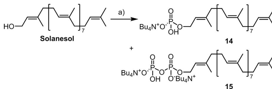
**Scheme 3.** a) Tetrabutylammonium dihydrogen phosphate,  $\text{CCl}_3\text{CN}$ ,  $\text{CH}_2\text{Cl}_2$ , 1 h, RT, 33% for **14** or 14 h, RT, 27% for **15**.
