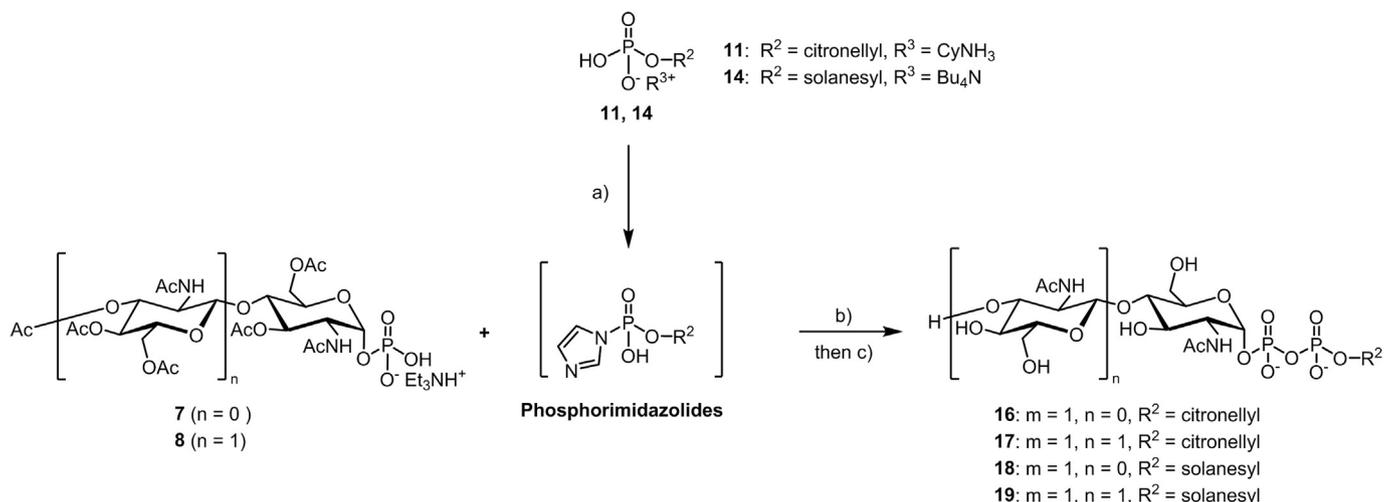
**Scheme 4.** a) i. Co-evaporation with Et<sub>3</sub>N and toluene; ii. CDI, THF, 1.5 h from **11** or CDI, CH<sub>2</sub>Cl<sub>2</sub>, 2 h from **14**. b) RT, THF, 12 h for **16**, RT, DMF, 12 h for **17**, RT, DMF, 6 days for **18**, RT, pyridine, 7 days for **19**. c) MeONa, MeOH, RT then DOWEX 50WX8, H<sup>+</sup> form.
