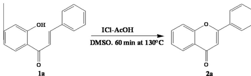
**Scheme 1.** Oxidative cyclization of 2'-hydroxychalcone to flavone.
