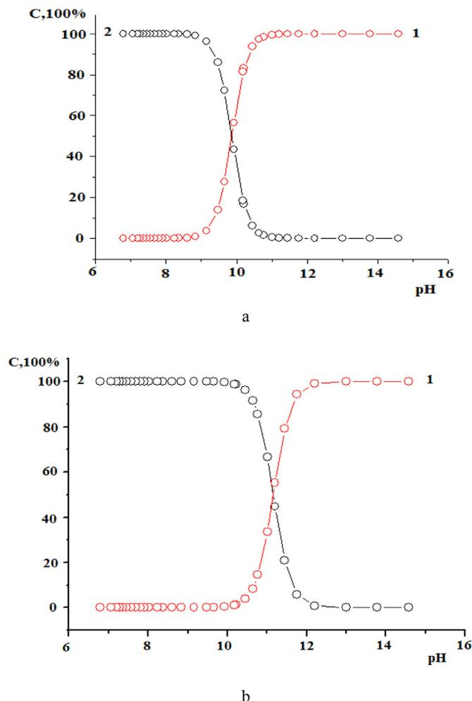
**Fig. 3.** Distribution of concentrations and spectra of the molecular (1) and doubly protonated (2) forms during the titration of compound (I) (a) and compound (II) (b).
