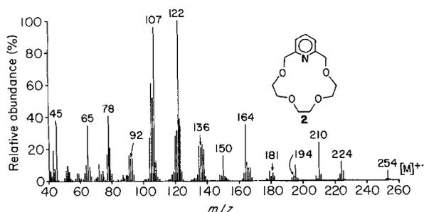
Figure 2. Mass spectrum of pyridyl-15-crown-5 (**2**).
