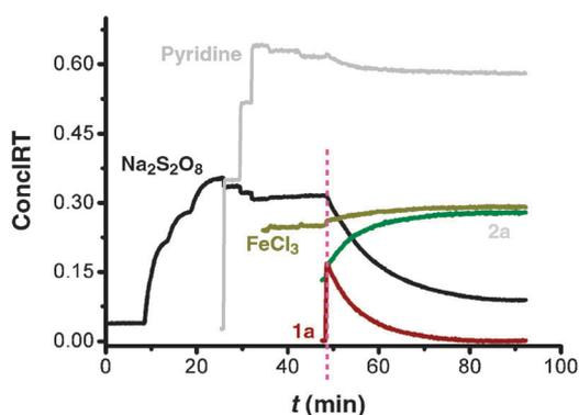
**Fig. 1** The 2D-kinetic profiles of the stoichiometric reaction of  $\text{Na}_2\text{S}_2\text{O}_8$  (0.2 M), pyridine (4 M),  $\text{FeCl}_3$  (0.02 M) and **1a** (0.2 M) added to 5 mL DMSO at 40 °C one by one; the reaction was monitored by *in situ* IR.
