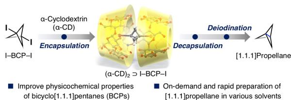
$\alpha$ -Cyclodextrin ( $\alpha$ -CD) encapsulation of bicyclo[1.1.1]pentane (BCP) derivatives could provide a bench-top-storable format for BCP derivatives. Furthermore, simple protocols for deiodination reaction of 1,3-diiodo BCP were developed to afford [1.1.1]propellane. Together, these findings provided novel and simple methodology for on-demand preparation of [1.1.1]propellane in a wide range of solvents (protic/aprotic/polar/non-polar) under mild conditions.
