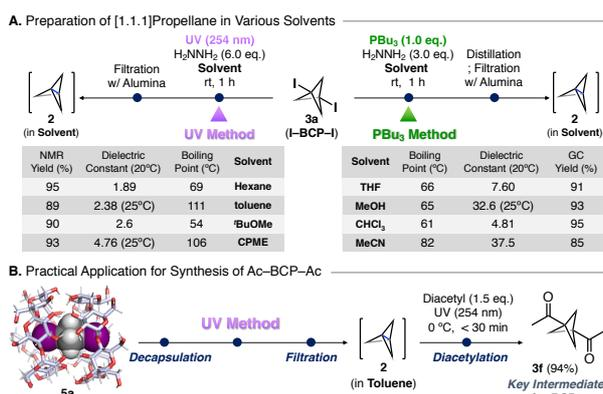
**Figure 5.** (A) Optimized protocols for preparation of [1.1.1]propellane. (B) Application for synthesis of Ac-BCP-Ac (**3f**) using a toluene solution of [1.1.1]propellane.
