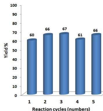
**Figure 5.** Recyclability test of  $A_1B_1$  in the model reaction of the N-formylation of morpholine: morpholine (1.0 mmol), phenylsilane (1.5 mmol),  $A_1B_1$  (1 mol%), dry THF (4 mL), room temperature, 24 h; GC yield using n-hexadecane as an internal standard.
