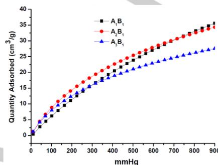
**Figure 4.** CO<sub>2</sub> adsorption isotherms at 273 K for A<sub>1</sub>B<sub>1</sub>, A<sub>2</sub>B<sub>1</sub> and A<sub>3</sub>B<sub>1</sub>.
