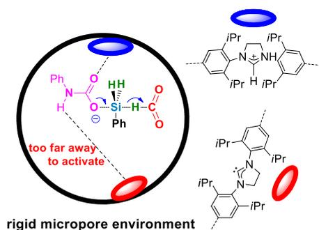
Figure 7. Proposed rigid micropore environment.
