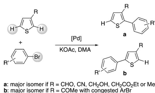
**Scheme 1.** Most reactive positions for Pd-catalysed direct arylation of 3-substituted thiophenes.
