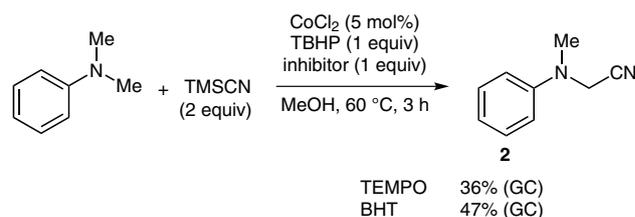
**Scheme 3** Control experiments with a radical inhibitor
