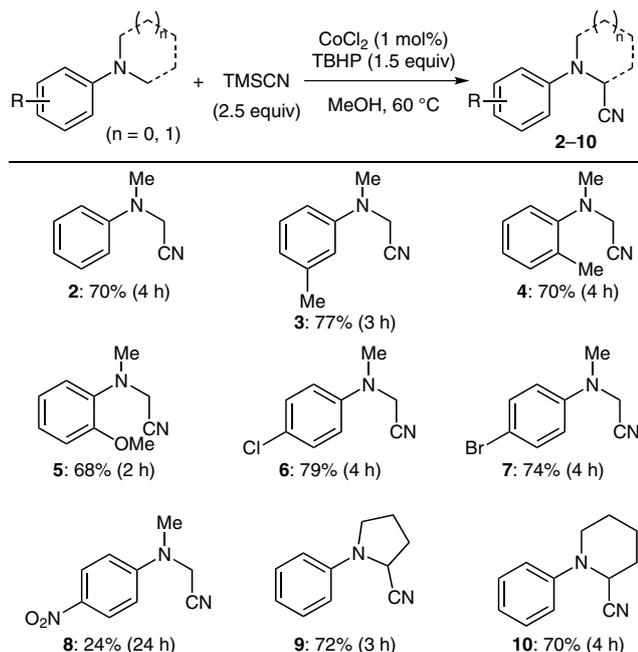
**Scheme 1**  $\text{CoCl}_2$ -catalyzed  $\alpha$ -cyanation of various tertiary aromatic amines; isolated yields are given
