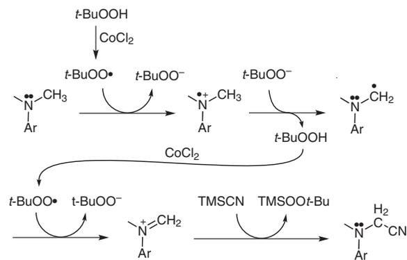
**Scheme 4** Plausible reaction path for cobalt-catalyzed  $\alpha$ -cyanation of tertiary aromatic amines with TBHP
