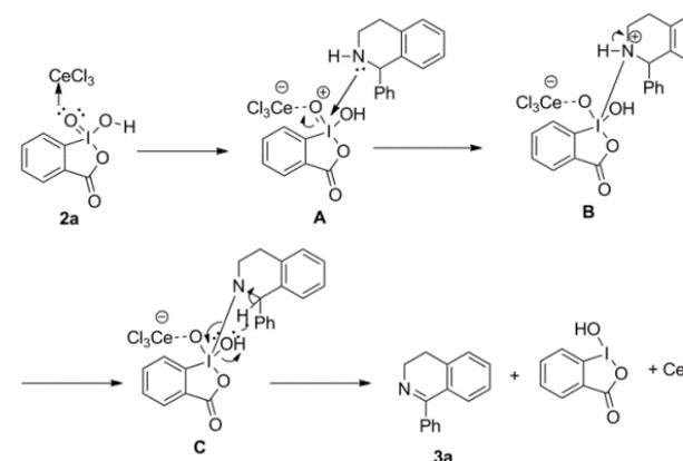
**Scheme 2.** Putative mechanism of oxidative dehydrogenation of 1-THIQs
