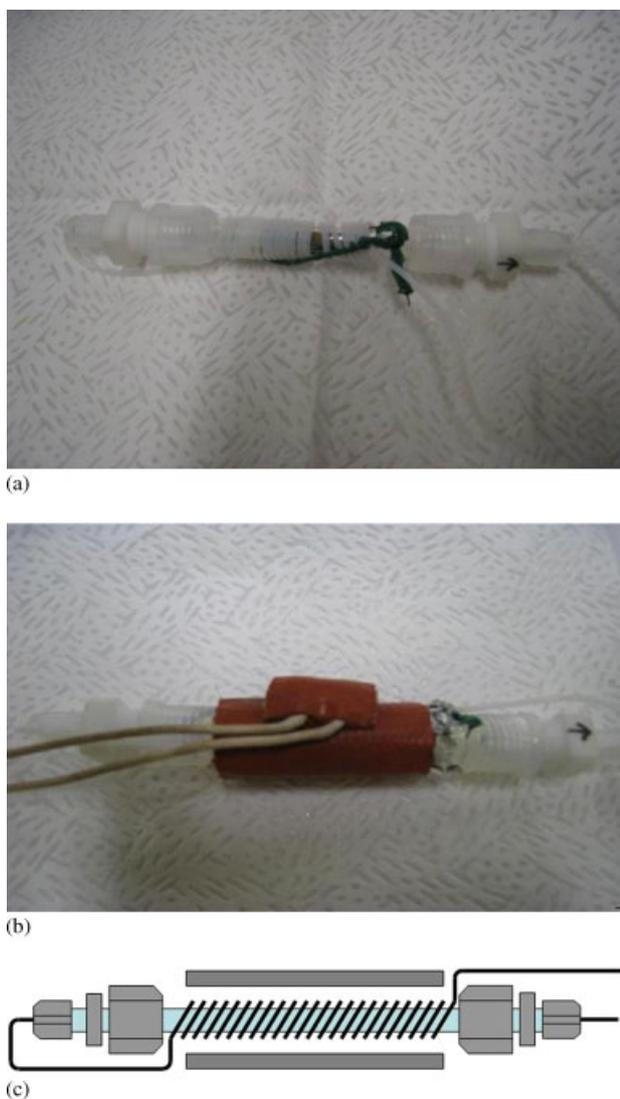
**Figure 2.** Pictures and a drawing of AgNO<sub>2</sub> column: (a) a glass column wound with a prior tube; (b) a glass column covered with foil and a rubber heater; and (c) a drawing of a glass column wound with a prior tube.
