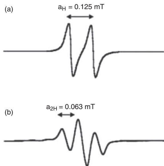
**Figure 8.** ESR spectra of (a)  $3^{2+}$  ( $5.0 \times 10^{-5}$  M) and (b)  $1a^{2+}$  ( $1.3 \times 10^{-4}$  M) in MeCN-CH<sub>2</sub>Cl<sub>2</sub> at rt.
