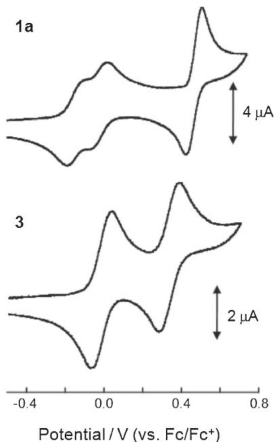
**Figure 2.** Cyclic voltammograms of **1a** and **3** in PhCN.**Table 2.** Redox Potentials of **1a–1c**, **2a–2c**, and **3**<sup>a)</sup>
