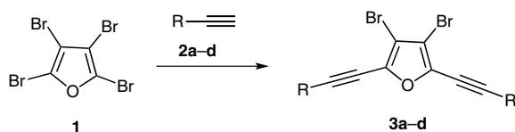
**Scheme 1** Synthesis of **3a–d**. *Reagents and conditions:* **1** (1.0 equiv), **2a–d** (2.4 equiv), CuI (5 mol%), Pd(PPh<sub>3</sub>)<sub>2</sub>Cl<sub>2</sub> (10 mol%), DIPA, 60 °C, 2 h
