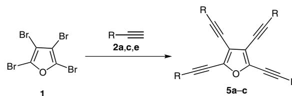
**Scheme 3** Synthesis of **5a–c**. *Reagents and conditions:* **1** (1.0 equiv), **2a,c,e** (4.8 equiv), CuI (5 mol%), Pd(PPh<sub>3</sub>)<sub>2</sub>Cl<sub>2</sub> (10 mol%), DIPA (5 mL), 75 °C, 2 h
