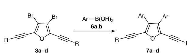
**Scheme 4** Synthesis of **7a–d**. *Reagents and conditions:* **3a–d** (1.0 equiv), **6a,b** (2.0 equiv), Pd(PPh<sub>3</sub>)<sub>2</sub>Cl<sub>2</sub> (10 mol%), K<sub>2</sub>CO<sub>3</sub> (3 equiv), dioxane, 70 °C, 2 h.
