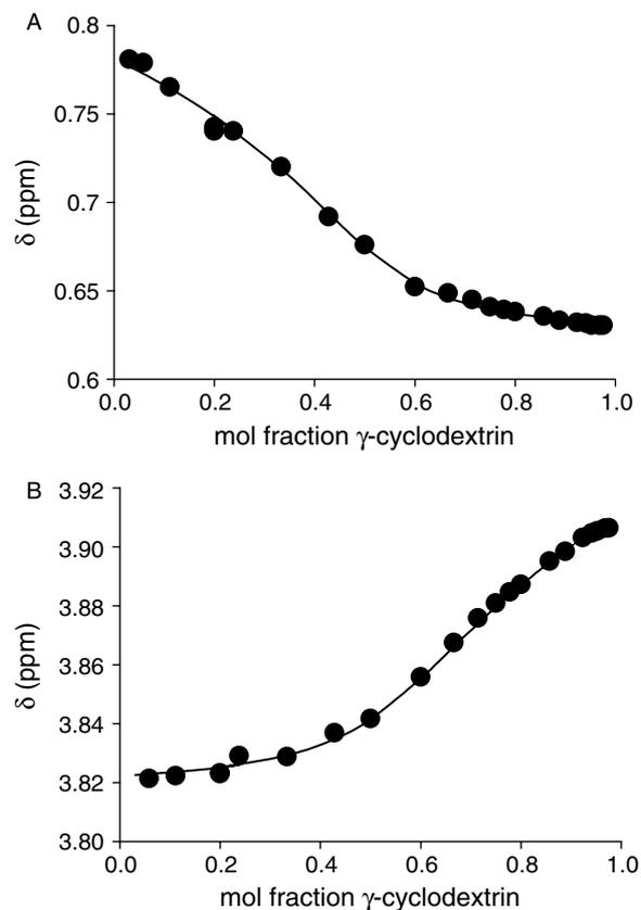
**Figure 2.**  $^1\text{H}$  NMR titration curves for Rocuronium Bromide with  $\gamma$ -cyclodextrin. (A) The behaviour of the steroid H-9 $\alpha$  proton signal. (B) The behaviour of the cyclodextrin H-3 signal. The points are the experimental data,  $[\mathbf{1}] = 0.41 \text{ mM}$  and  $[\mathbf{3}]$  ranging from 0.013 to 8.2 mM at 30 °C, and the solid line is the least squares fitted calculated curve using parameters from Table 1.
