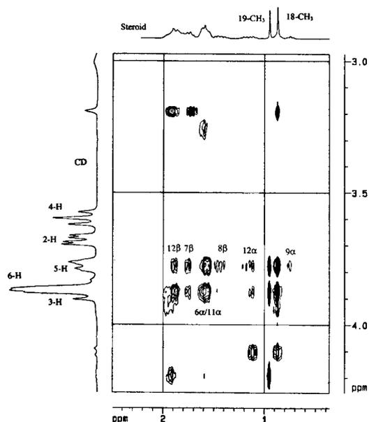
**Figure 8.** A section of the ROESY spectrum of Org 7042 (6 mM) and  $\gamma$ -cyclodextrin (6 mM) showing clear correlations between the steroid protons and the cyclodextrin protons H-3 and H-5.
