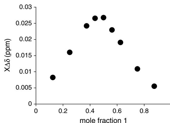
**Figure 5.** Job plot for the fast exchange system, Rocuronium Bromide and Org 25969 at pH 9.1, 70 °C. The total concentration  $[\mathbf{1}] + [\mathbf{3}] = 1.0 \text{ mM}$ .
