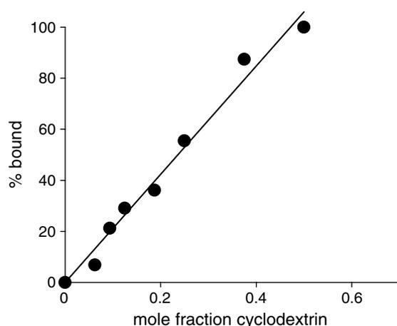
**Figure 4.** Binding isotherm for the slow exchange system, Rocuronium Bromide with Org 25969 at pH 7.5, 30 °C.
