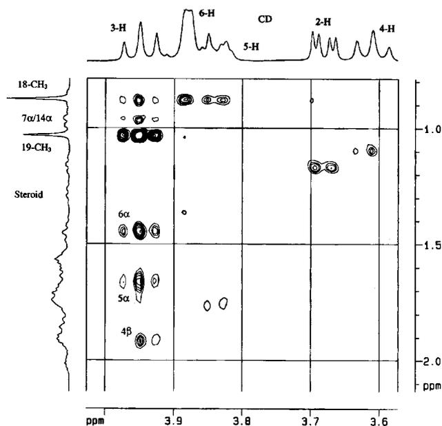
**Figure 7.** A section of the ROESY spectrum of Org 7042 (6 mM) and  $\beta$ -cyclodextrin (6 mM) in pH 7.6 buffered  $\text{D}_2\text{O}$  showing strong correlations between the steroid and the H-3  $\beta$ -cyclodextrin proton, and weaker correlations to H-5.
