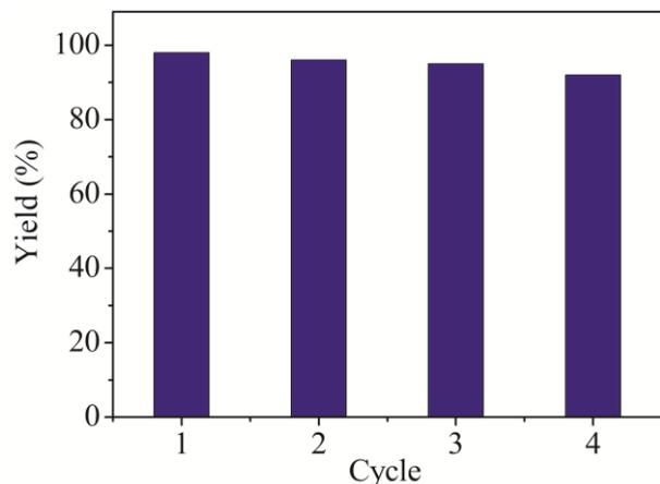
**Figure 4.** ZnO/RGO catalyst recycling.
