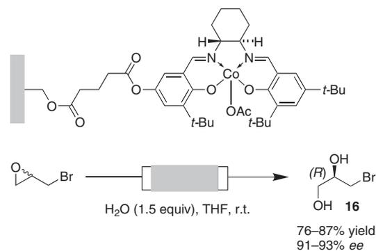
**Scheme 5** Dynamic kinetic resolution of epibromohydrin under continuous-flow conditions using a PASSflow microreactor.
