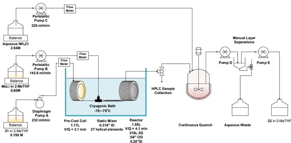
**Figure 1.** The process flow diagram of the experiment with continuous quench and phase separation.
